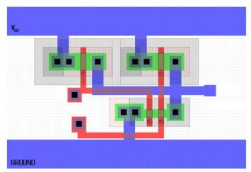
NAND2. The pull-up network has two PMOSFETs in parallel and the pulldown network has two NMOSFETs in series. Interestingly, we can see that the designer didn't balance tphl and tplh.
